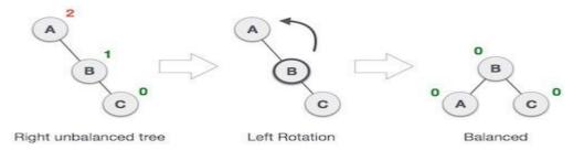
In our example, node **A** has become unbalanced as a node is inserted in the right subtree of A's right subtree. We perform the left rotation by making **A** the left-subtree of B.
