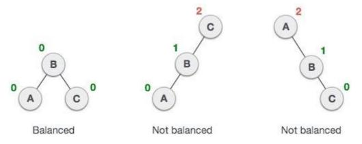
In the second tree, the left subtree of **C** has height 2 and the right subtree has height 0, so the difference is 2. In the third tree, the right subtree of **A** has height 2 and the left is missing, so it is 0, and the difference is 2 again. AVL tree permits difference (balance factor) to be only 1.
