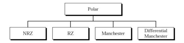
Polar encoding uses two voltage levels (positive and negative).
