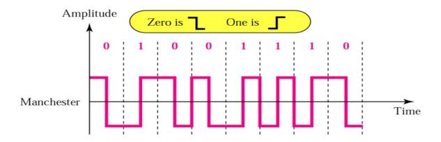
In Manchester encoding, the transition at the middle of the bit is used for both synchronization and bit representation.
