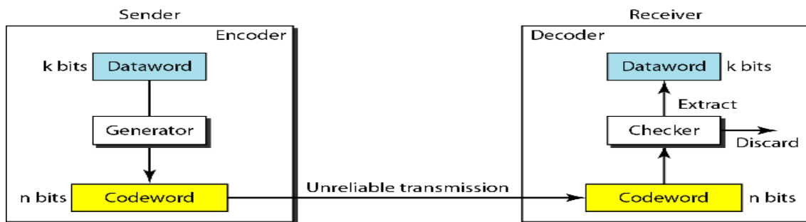
Figure: Process of error detection in block coding
