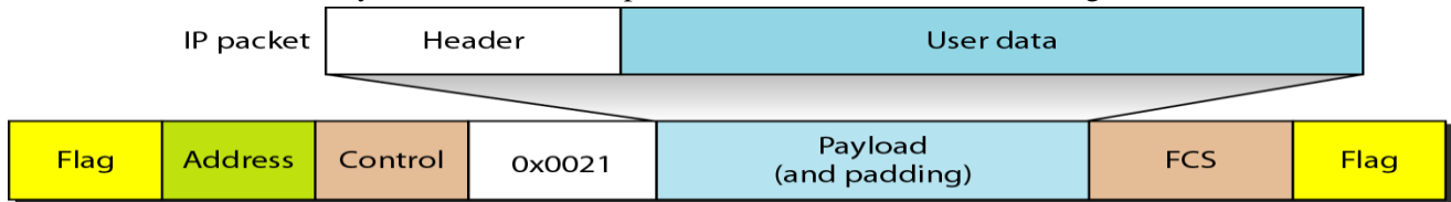
Figure: IP datagram encapsulated in a PPP frame
