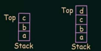
A Pushdown Automata (PDA) is a way to implement a Context Free Grammar in a similar way we design Finite Automata for Regular Grammar
