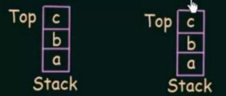
A Pushdown Automata (PDA) is a way to implement a Context Free Grammar in a similar way we design Finite Automata for Regular Grammar
